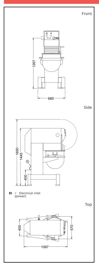
Electric 220-240/380-415 V/3 ph/50 Supply voltage: Electrical power, max: 1.54 kW **Total Watts:** 1.54 kW Capacity: ISO 9001; ISO 14001 kg/ Performance (up to): Cycle Capacity: 60 litres Key Information: External dimensions, 685 mm Width: External dimensions, Depth: 1087 mm External dimensions, **Height:** 1445 mm **Shipping weight:** 330 kg
